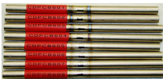
Figure 13. Special Specimens. Set of 8 specimens of kind “1” (Table 1) to investigate late welding after pickling and cleaning the titanium samples.
